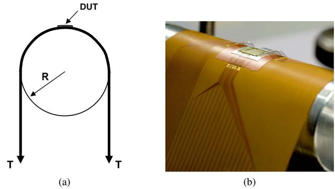
Fig. 4. Thin-film chip bending (a) The principle: thin-film DUT on foil bent under defined radii ( $R$ ), (b) Apparatus: cylindrical deformation
