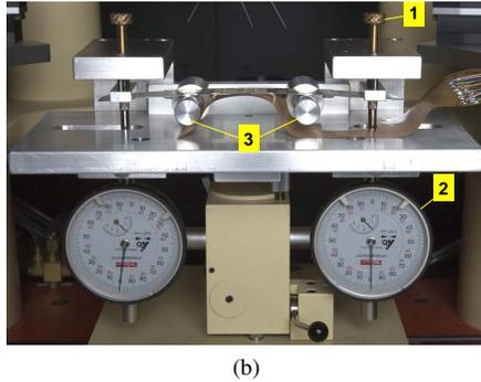
Fig. 2. (a) 4-point bending technique, (b) Bending apparatus
