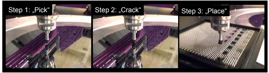
Fig. 7 Snapshots from a video illustrating the Pick, Crack & Place™ process.
